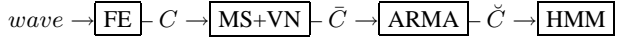
Fig. 1. Block diagram of our feature post-processing technique. Abbreviations are : FE – feature extraction; MS – mean subtraction; VN – variance normalization; ARMA – mixed auto-regression and moving average filter; and HMM – hidden Markov model, the standard backend for training and decoding.
